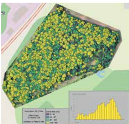
Computer code can be used to predict crown boundaries and provide statistical information across the whole stand.
